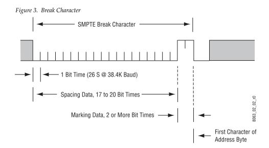
The break forces all *tributaries*, or listeners (such as the switcher's editor port), from the "Idle" state into the "Active" state. A break can be sent only by the Edit Controller. When the switcher receives the break, it ceases all bus communications, resets any communication error condition, and prepares to receive an address (Figure 4).
